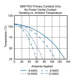
NOTE: Temperature rise charts are based on 25 °C ambient temperature.
